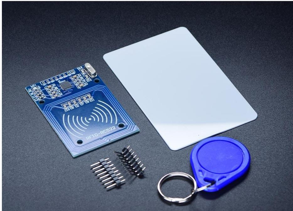
Fig 2.9: RFID Reader and Tag
