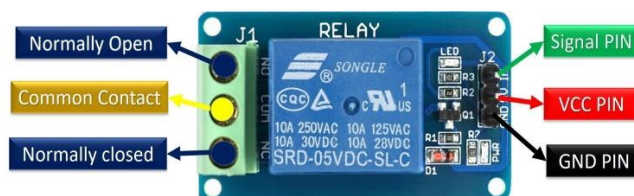
Fig 2.4 Pin Configuration of Relay Module
