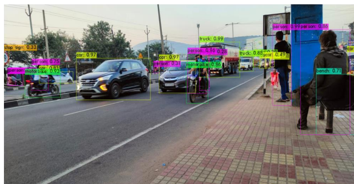
Fig: 6.1 Object detection using yolo v3
