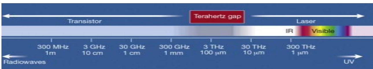
Fig.1.4 Terahertz frequency range.
