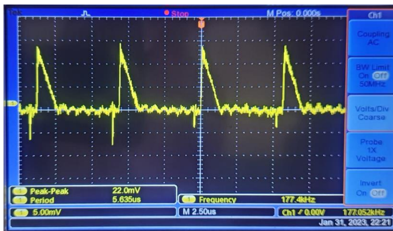
Fig 3.5- Dual Power Supply without Liner Regulator
